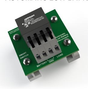
The Rugid Computer SMART SWITCH is an automatic low battery disconnect. The Smart Switch is designed to work with any 12 VDC control panel or power supply. To prevent a deep discharge of a battery during an extended power outage, the Smart Switch will automatically disconnect the battery when the voltage falls below the user adjustable cutoff voltage. When power is restored the Smart Switch will automatically reconnect the battery.
